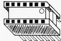
We made a special purchase of PC mount solder tail sockets, including discontinued types and some that need higher than spec insertion force. Brand new from a leading manufacturer of quality IC sockets.
