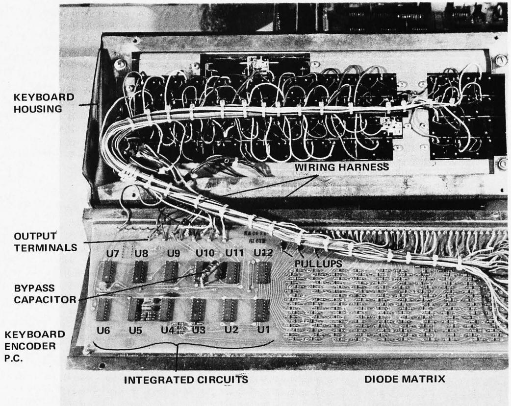
keyboard of the 1966-1970 vintage. This keyboard is a surplus Sanders Associates Model 722-1 subsystem, which comes enclosed in a metal housing with a fairly typical Teletype style key layout. On the right hand side of the keyboard is a set of special function keys, which obviously had some meaning in the original system using the device.
