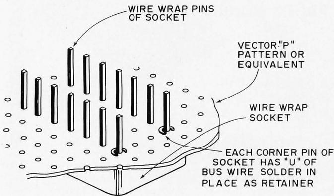
If you want to wrap up a quick project, it is often handy to use perforated board (eg: Vector "P" pattern VECTORBOARD) to mount wire wrap sockets. I have used many methods for attaching boards — rivets, bolts, epoxy glue, cyanoacrylic glue, etc. One method which I dreamed up the other day to solve the mounting problem for a small test jig may prove useful to you at some point. Simply put the socket through the perforated board, then solder each corner pin with a "U" shaped retainer made of bus
