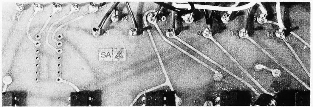
the positive supply and ground, with markings of (+) for the supply side and (-) for the ground side. In the disassembled keyboard photograph accompanying this article, the bypass capacitor is labeled. Using clip leads, the bypass capacitor often provides a handy way to apply power when first testing the board.
