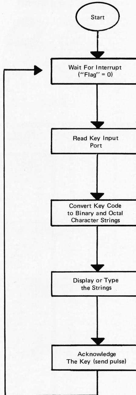
Fig. 6. Keyboard Test Program Flow Chart.
